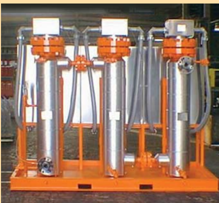
480 kW boiler water pre-heater
