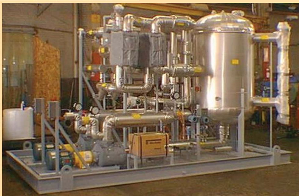
The above photo shows a 550°F hot oil system during the final operating test.
