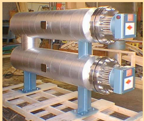
80 kW steam superheater
