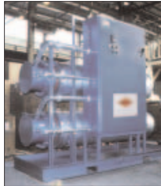
This 80 kW multiple chamber assembly preheats fuel oil.
